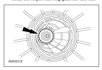
23. CAUTION: Always install a new output shaft retaining ring.
